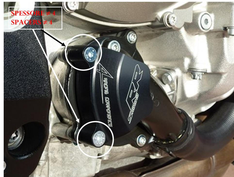
After removing the original screws applied on covers that taking notice to fit the shims under it in the locations indicated.
